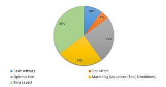
Fig. 8. Time necessary to create of an NC program with NC strategies
