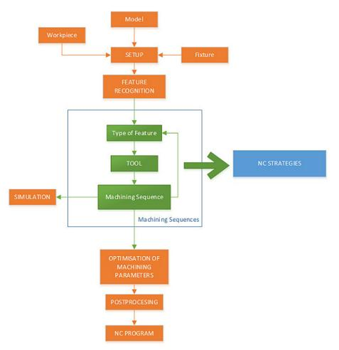
Fig. 6. The process of creating the machining process in CAD/CAM system Edgecam 2016 R2
